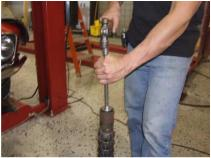
10. Once that is complete you need to make sure the steering shaft itself is clean and free of burs. Install the supplied bearing over the steering shaft and tap it into the column tube by walking it in with a small hammer.
