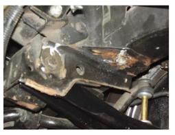
10. Once the bracket is installed you can now connect your outer tie rods to your steering arms. Note the kit has been shipped to you with 2 sets of tie rods. You need to determine which ones you use by comparing the taper size of your stock tie rod. Be sure that the tie rod you select fits your steering arm tightly and locks on the taper.
