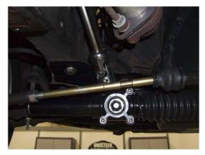
11. Next, you need to modify the column and tube assembly. Using a band saw or a Sawzall, cut off the rag joint as close to the weld as possible. Once that is done, clean the steering shaft of rust and scale. Install supplied bearing over shaft and into column tube. Tap the bearing in with a small hammer until seated in the column. Measure down 1 ¾ inch from the flat surface of the bearing. Mark the shaft and cut on the line.
