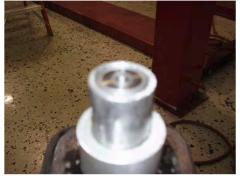
14. Next install the u-joint over the steering shaft. Using the supplied drill bit and the pilot hole in the u-joint drill through the pilot hole and clear through the other side of the u-joint.
