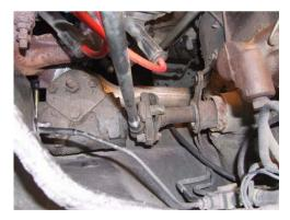
6. Once the column is out of the car, do the following. In a band saw or using a Sawzall cut the steering shaft off as close to the weld of the rag joint as you can.
