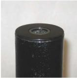
12. Install supplied brass washer and u-joint. With both of these pieces installed, make sure there is not a gap between the lip of the bushing and the end of the steering column.
