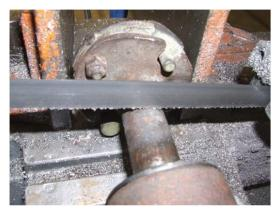
7. Next, you need to cut off the inner tube of the steering column tube. (This is the tube that has the lever on it.) Cut it off as close to the steering column tube as you can. DO NOT CUT THE ACTUAL STEERING COLUMN TUBE. When cutting the inside tube, be sure to only cut the tube itself and not the inside steering shaft. You can accomplish this by going around the tube with your saw.
