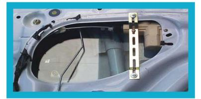
Notice how this actuator is partially fastened to the door and to the strap. You should be  $\Box$ clear on the fact that the attachment is not  $\Box$ as critical as the placement. Just make sure that the actuator is attached securely, and does not interfere with any other mechanism. Whenever installing an actuator inside the metal panel, extreme care should be taken with regards to window movement.
