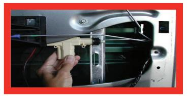
This photo shows placement of the actuator  $\Box$ in position prior to fastening. The vehicle in  $\Box$ the photo is a 2000 Chevy Silverado. Photos and installation compliments of A-1 Electric. A-1's installer will use the strap that is supp- $\Box$ lied in the Electric-Life door lock kit to span□ the hole in the door and permanently fasten  $\Box$ the actuator in place.
