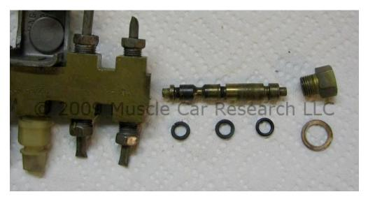
Inspect the bores once the pistons have been removed. If the bores aren't perfectly smooth you should either replace the affected valve body or have the bores professionally sleeved.
