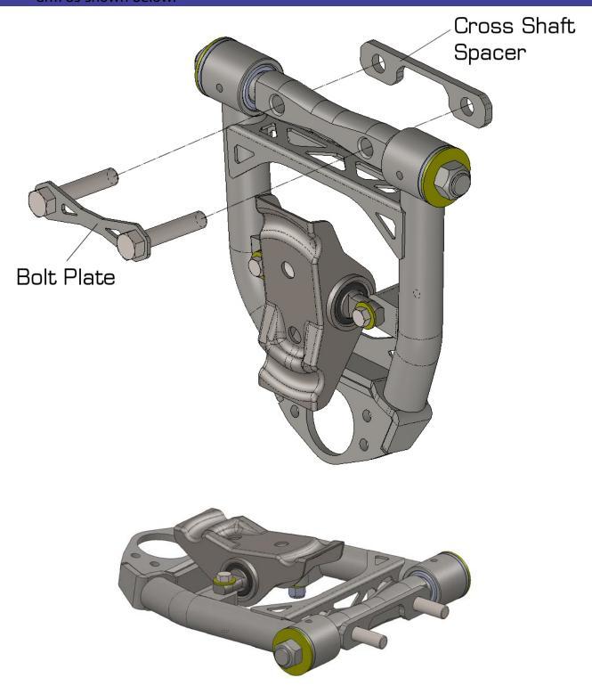
Install the arm onto the vehicle. Do not worry about using alignment shims at this point. You will need to align the vehicle after the installation is complete anyways. Fasten the bolt plate using the provided washers and nylock nuts. Repeat the steps 1-7 in reverse order to complete the install.
