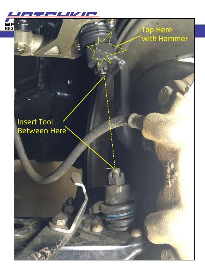
All that is left holding the upper control arm to the car is the goss shaft fasteners.
