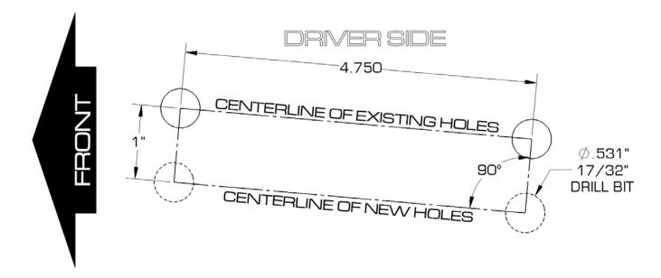
Basically the new bolt pattern is 1" down. This dimension are orthogonal to the centerline of the existing holes.
