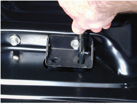
Marking center with drill bit
