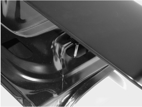
Aligning wing to underside of deck lid.
