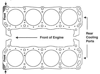
**TO INSURE PROPER COOLANT CIRCULATION**, the word FRONT is stamped on both sides of the head gasket and must always be installed towards the front of the engine.
