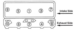
**Intake Manifold:** Using a torque wrench, torque all bolts to 23-25 ft. lbs. **DO NOT EXCEED** torque specifications.
